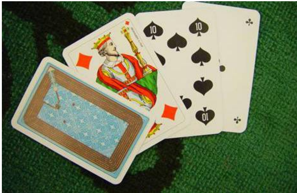
3.1 Smart Playing Cards. These ordinary playing cards are made “smart”, or computationally enhanced and network-capable, through Radio Frequency Identification (RFID) tags attached to the backs of the cards. (Distributed Systems Group, 2005)
